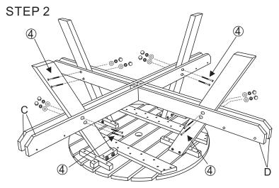
Fix two pieces cross brace C of table leg A and two pieces cross brace D of table leg A by using 8 sets of bolts, washer , nut and hat 4. Note the difference of part C and D. ① = 8pcs 4 = 8pcs reference the drawing.
